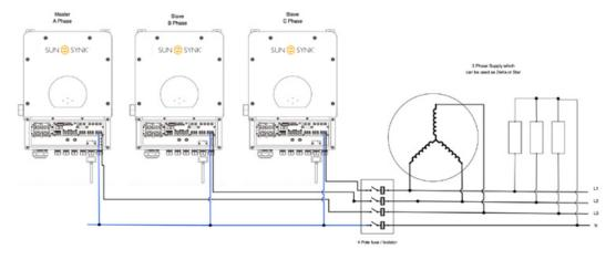
For stability, all the batteries need to be connected in parallel. It is recommended a minimum cable size of 50mm diameter with fuse isolators to each inverter.
